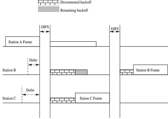
Fig. 1. IEEE 802.11 backoff mechanism
