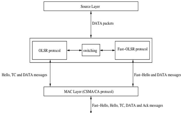
Fig. 7. The generic Fast-OLSR scheme in our simulation
