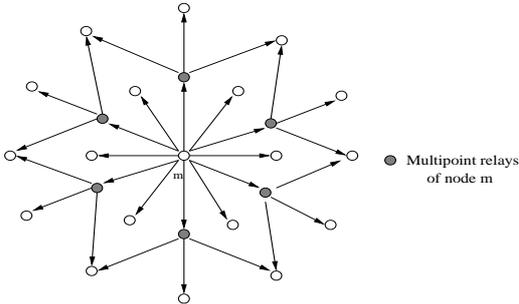
Fig. 2. Multipoint relays of node  $m$
